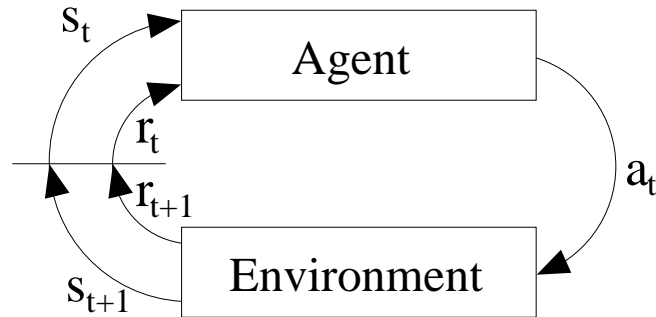
Figure 2.1: The cycle of sensing the environment, acting and receiving a reward in reinforcement learning agents. The agent receives situation s_t and reward r_t at time t and answers with action a_t , which leads to a new situation s_{t+1} and reward r_{t+1} .
